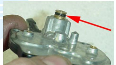
1.7 (Below) Remove the o-ring from the circuit chamber. Remove the two screws securing the high-speed circuit to the chamber and remove the plate. Remove the gaskets and film-valve.
