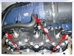
3.6 (Below) Remove the two 12mm bolts securing the stinger pipe to the head.
