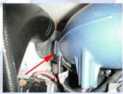
3.5 (Below) Remove the head and pipe water cooling lines.
