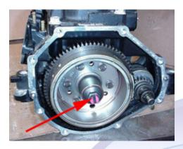
5.3 (Below) Use a universal flywheel puller to remove the flywheel from the shaft. Do not ship the flywheel key to SBT.
