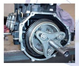
5.4 (Below) Pull the starter bendix out of the housing.
