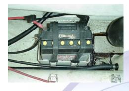
1.1 (Above) Remove the two retaining straps, disconnect the battery and remove it from the hull. Disconnect the negative (black) cable first, then the positive (red).
