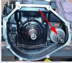
5.5 (Below) Remove the remaining 10mm bolt from the starter and pull it back out of the flywheel housing.
