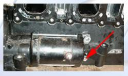
5.6 (Below) Remove the pulse lines from the case.
