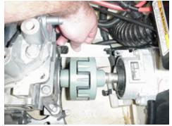
Take a small straight edge and place it on the coupler. You are looking for an even match all the way around the coupler. Place shims where necessary to align the couplers.
