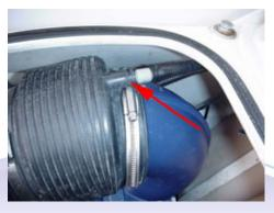
3.4 (Below) Loosen the waterbox coupler with a screwdriver and pry off the rubber fitting from the stinger pipe.
