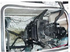
4.5 (Below) Remove them with a 14mm socket and remove the supports.
