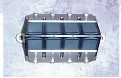
2.12 (Below) Look at each petal-to-cage surface and check for gap. If a gap of more than 0.015" is present, replace the petals.
