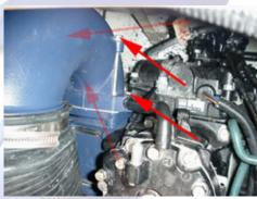
3.7 (Above) Using a 12mm socket, remove the four 12mm bolts securing the exhaust pipe to the exhaust manifold. Wiggle the pipe towards the front of the boat and pull it up and out of the hull.
