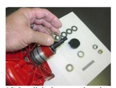
15). Install the larger steel washer (14) first then apply a thin later of the provided grease (22) to the shaft. This will act as an adhesive to hold the needle bearings (15) to the shaft as you install all 40 of them (count them 40).
