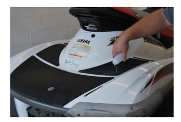
Give it a few minutes to work, then begin pulling upwards on the mat edge as you scrape between the mat and fiberglass to work the mat free. As you loosen sections of mat, continue the process, applying the adhesive remover, letting it soak in, and then lifting and scraping.
