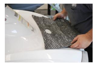
All BlackTip Jetsports mats come with peel-and-stick adhesive; others require contact cement. If your set is the latter, make sure the adhesive you choose is waterproof, and that you follow the manufacturer's directions. Typically this means coating both the footwell and the underside of the mat with adhesive, letting it dry till it becomes tacky, and then pushing the pieces together.
