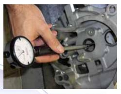
Subtract the crank journal 1.4 measurement from the bearing ID measurement for each location and note the resulting clearances. If the results are not between 0.001" - 0.002", reassemble the case with the appropriate over/under size bearings to create the correct clearances.
