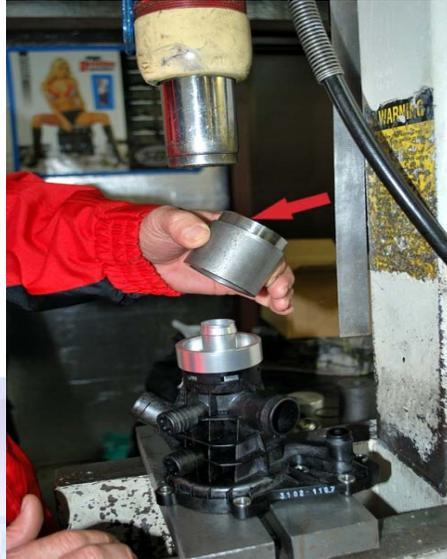
This is how the retaining ring gets seated on the press.
