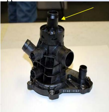
2) Use a piece of scrap block and install the steel tab cutter down around the original flange of the plastic housing. Press down to cut the plastic tabs that hold the thermostat housing outlet nipple. The metal cutter will shear the tabs so you can remove the old thermostat.
