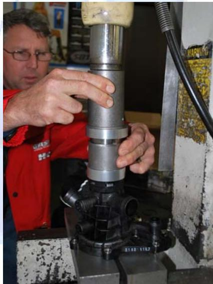
Now your thermostat housing is finished and can be reinstalled onto the engine.
