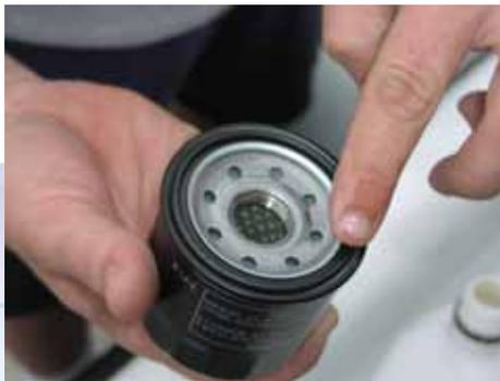
3.2 (Below) Install the new filter, tighten to hand tight. Fill the oil reserve with the same amount that was removed (check the suction pump). You should be able to get 4.5 quarts out.
