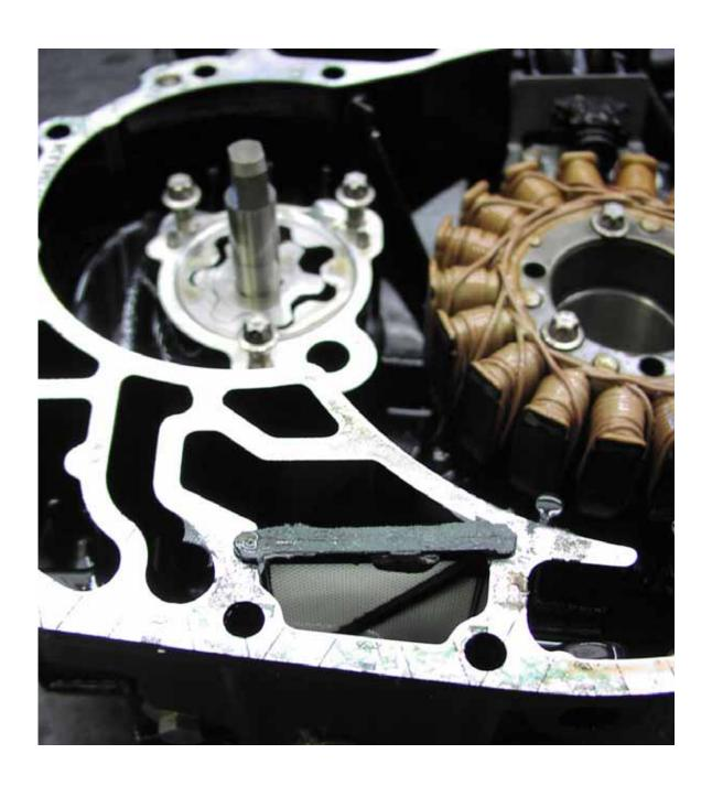
Damaged rotors, cover and guides:
