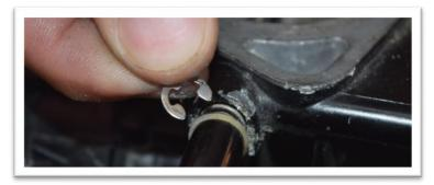
c. Slide the shaft(s) out of carb(s). Sometimes they can be difficult to remove. Use penetrating spray lube if needed.
