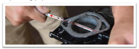
3. Insert the provided brass fittings into the holes left by choke shaft(s) absence. Each carb will have two holes, one on each side of the throat. One hole gets a plug, the other hole gets a nipple. Your application dictates which side will have a plug or nipple.
