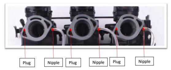
4. Plumb the tubing like the diagram shows below. Leave enough slack to mount the plunger where you want it. If you have a double or single carb, split the lines accordingly using the provided <u>plastic T's</u>
