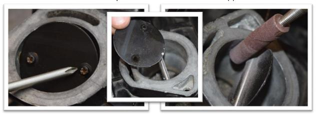
b. Remove all the E-clips located along the choke shaft using a pick or a small flathead screwdriver.
