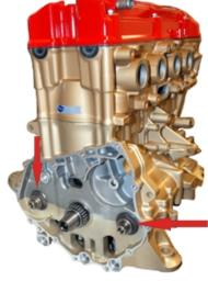
The oil pan should be left intact with all bolts. This is for the N/A & Turbo models.
