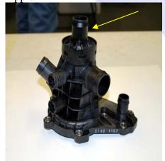
2) Use a piece of scrap block and install the steel tab cutter down around the original flange of the plastic housing. Press down to cut the plastic tabs that hold the thermostat housing outlet nipple. The metal cutter will sheer the tabs so you can remove the old thermostat.
