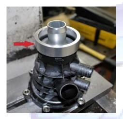
6) With the cutting edge facing up on the tab cutting tool and a piece of scrap wood or aluminum between the cutting tool and the press, begin pressing down. Take your time and allow the edge of the plastic housing to meet the inside lip on the aluminum retaining ring.
