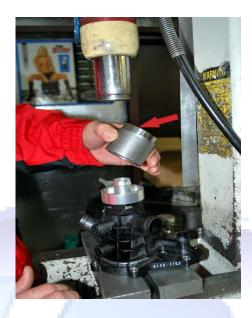
This is how the retaining ring gets seated on the press.
