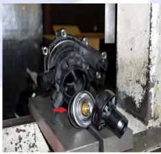
Notice the red arrow shows that the o-ring is on top of the thermostat.
