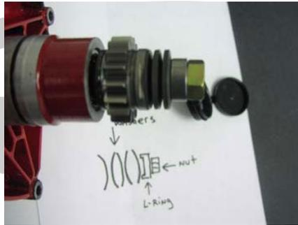
20). Install the L-ring (19) and hex nut (20) (use blue locking agent). Torque nut to **22ft-lbs.**- make sure to hold the locking washer with the retaining wrench provided in the Supercharger tool kit.
