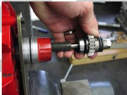
3). Use the 4 pin spanner socket to remove the retaining disk and push the bearing that is located behind the disk out of the housing. It pushes out towards the disk you removed.
