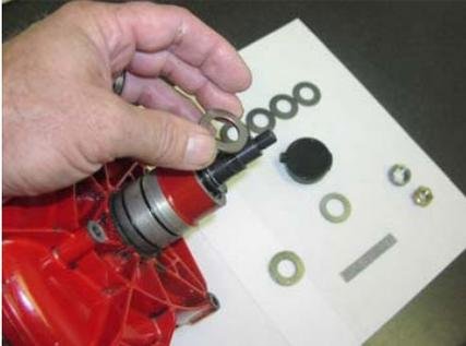
15). Install the larger steel washer (14) first then apply a thin layer of the provided grease (22) to the shaft. This will act as an adhesive to hold the needle bearings (15) to the shaft as you install all 40 of them (count them 40).
