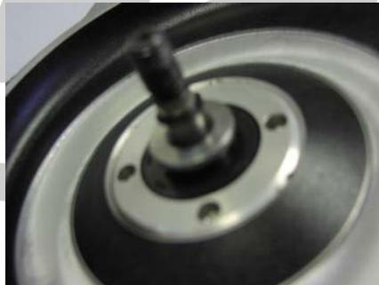
12). Install impeller turbine, then washer (4) and cap nut (3) –use blue thread lock agent torque to 22ft lbs. **Note: This is left handed threads.** You can hold the shaft from turning temporarily installing the new locking washer on the other end of the shaft and holding it with
