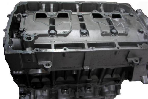
Figure 2: Oil pan covers removed.
