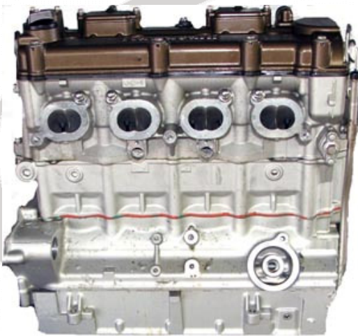
Figure 6: Intake side of the motor.
