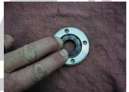
6). Install one of the new bearings into the supercharger housing using the bearing install tool, then screw the retaining disk (9) back into the housing. Torque this part to 22 ft-lbs.
