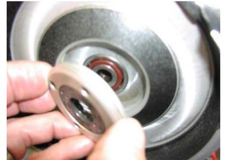
4). Clean off any old gasket material and dirt that is on the housing sealing surfaces before re-assembly.
