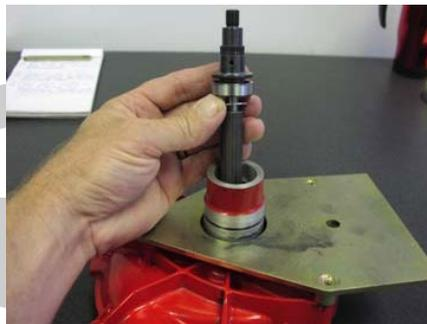
11). Install the step collar (7) and o-ring (5) to the inside section of the Supercharger. (photo below)
