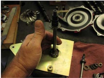
(8). Tap the shaft lightly with a block of wood and a mallet to seat the bearing down and into position.
