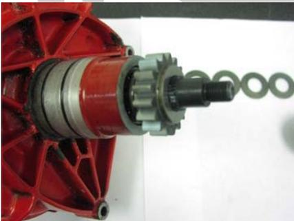
17). Slide the other steel washer (16) up over the shaft, then install the locking washer (17) with the two flat spots for the wrench to hold.
