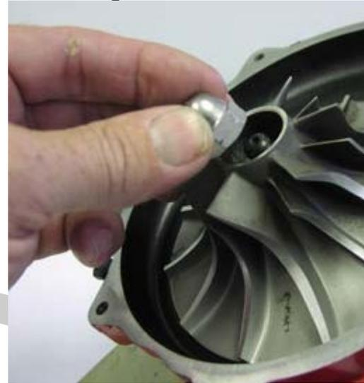
13). Use black high temp sealant to re seal the housing halves and blue thread lock on the bolts holding the housing together. Torque to: **89 inch-pounds not ft pounds.**
