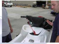
4.2 (Below) Check the dipstick to verify correct oil level. On a cold engine set the level to the lower ½ of the marker range. A hot engine should be in the top ½.
