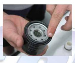
3.2 (Below) Install the new filter, tighten to hand tight. Fill the oil reserve with the same amount that was removed (check the suction pump). You should be able to get 4.5 quarts out.
