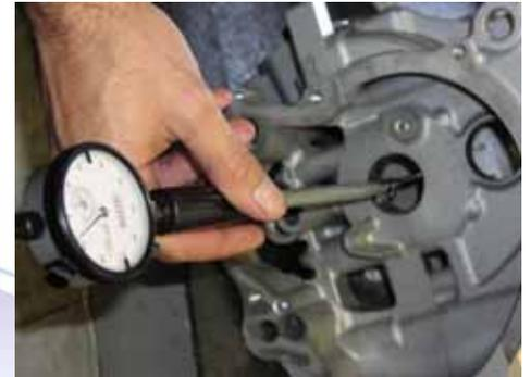
1.4 Subtract the crank journal measurement from the bearing ID measurement for each location and note the resulting clearances. If the results are not between  $0.001''$  -  $0.002''$ , reassemble the case with the appropriate over/under size bearings to create the correct clearances.
