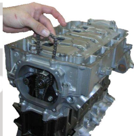
Figure 3: Timing chain is left inside of engine.
