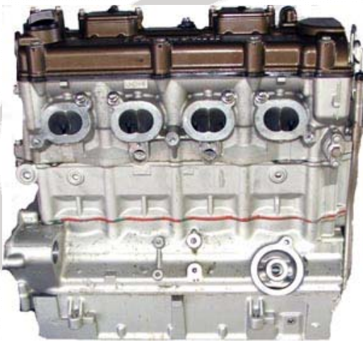
Figure 6: Intake side of the motor.
