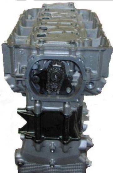
Figure 1: Oil Pan cover is removed.
