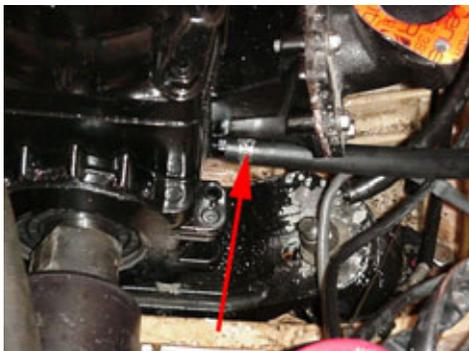
4.2 (Below) Remove the 13mm bolt from the rear of the exhaust at the bracket.
