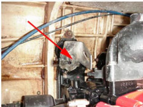
5.4 (Below) **NOTE: DO NOT CUT THE WIRES!** Disconnect all the wires coming through the grommet into the box. Note the location of the wires connected directly to the circuit board for later installation. All other wires are color coded. Remove the two Allen head bolts & grommet from the box then pull the wires through and out.
