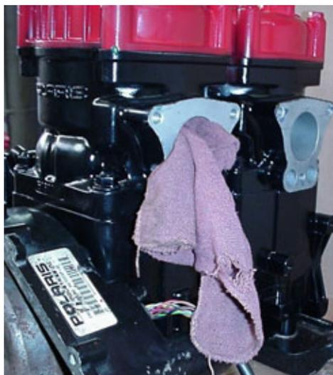
6.7 (Below) Remove the seven 10mm bolts securing the flywheel cover and remove it.
