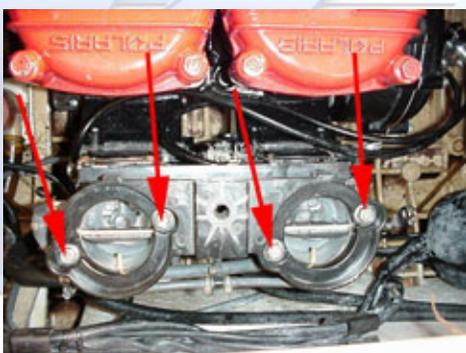
3.3 (Below) Remove the throttle, oil pump and choke cables from the carburetor assembly. Pivot the shafts for easy removal of the cable end-barrels.
