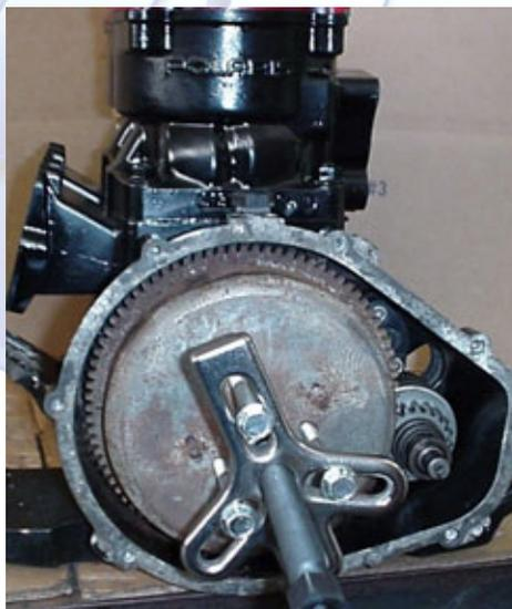
6.10 (Below) Remove the two 10mm bolts securing the starter to the case.
