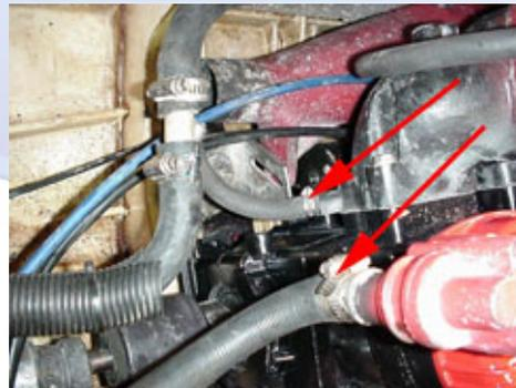
4.5 (Below) Remove the top Exhaust bolts with a 19mm socket and wrench. Remove the pipe from the hull.
