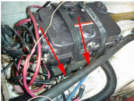
1.1 (Above) Remove the two retaining straps, disconnect the battery and remove it from the hull. Disconnect the negative (black) cable first, then the positive (red).
