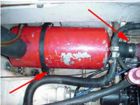
4.3 (Below) Remove the pipe and manifold cooling inlet and exit lines.
