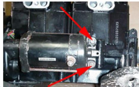
6.11 (Below) Remove the three screws securing the stator and swing it aside to gain access to the flywheel housing bolts. Remove the four 13mm bolts securing the flywheel housing to the case and remove the housing.
