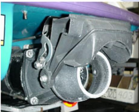
2.2 (Below) On the back of the pump assembly, the reverse gate rod (if equipped) and steering rod need to be removed. The steering rod nut can be removed using a 9/16" wrench.
