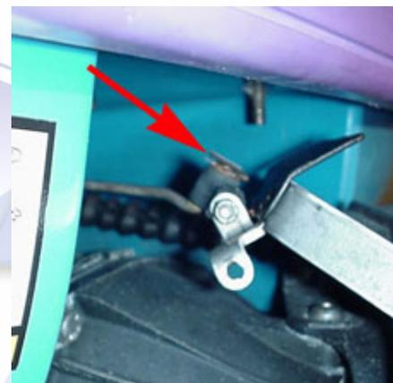
2.4 (Below) On the inside of the hull, at the rear, the cooling water intake and bilge hoses need to be removed. Loosen the hose clamps with a screwdriver, then work the hoses off the nipples.
